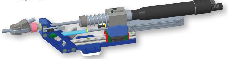
BTS-R-50 can be integrated in a UR10E and with our own UR-CAP the system can quickly be deployed as the basic programming and Run Routines are all ready in our CAP. Similar Software are also prepared for AUBO Collaborative robots for your convenience.
